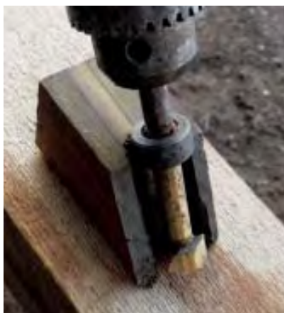
Figure 13. Use the angle obtained with the speed square to make an angled block to guide the drill on stair newels. The block is cut on a miter saw. Here, the carpenter is preparing to drill the large diameter side of a two-step hole for a cable stud.
